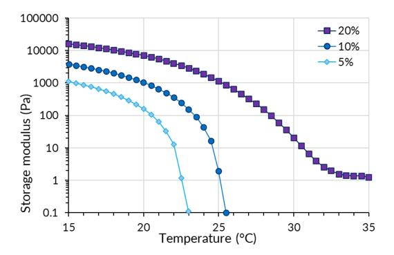
**Figure 1.** Decrease of storage modulus for GeIMA hydrogels at various concentrations over an increasing temperature.
