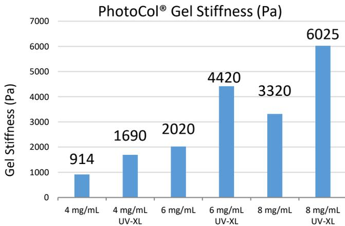
\*Rheology testing was done on a Bohlin CVO-100 rheometer. Crosslinked collagen was exposed to 365 nm UV light for 5 minutes.
