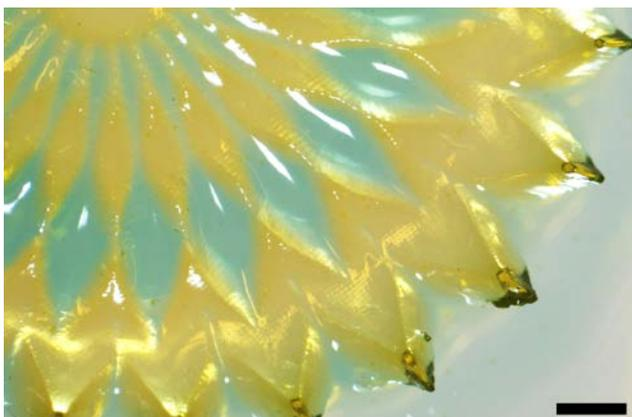
Figure S3: Flower-like structure printed via DLP (stained in yellow), with hollow spaces and channels in between the petal-like structures. These channels are infused with a second hydrogel (stained in blue). Scale bar is 500 $\mu$ m.
