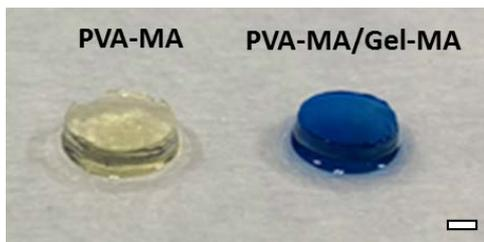
Figure S2: PVA-MA and PVA-MA/Gel-MA hydrogels post 12 hours incubation in Coomassie plus reagent. Scale bar = 1mm.
