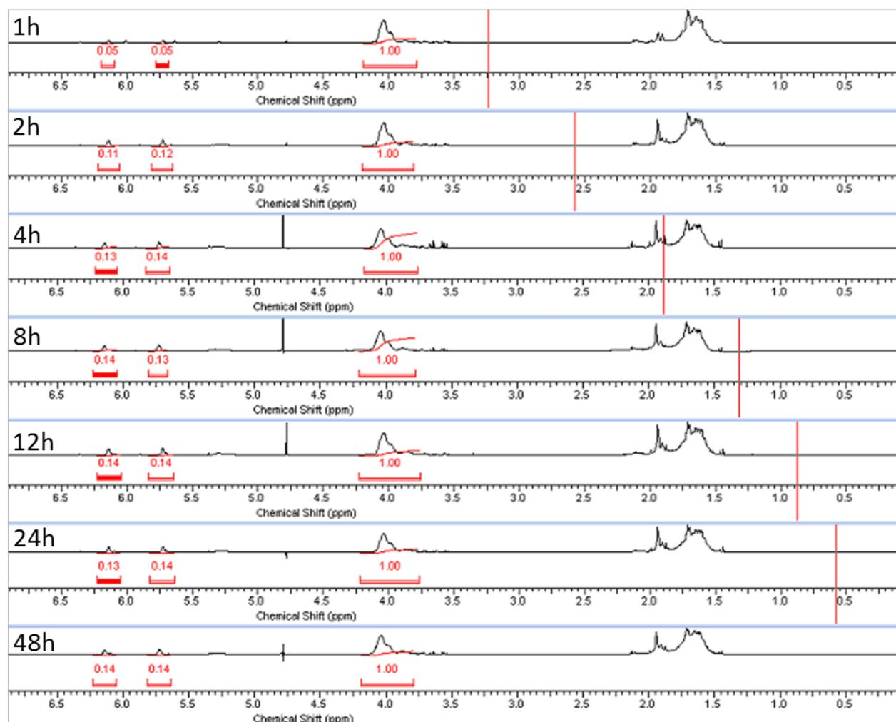
Figure S1:  $^1\text{H-NMR}$  spectra of PVA-MA and the respective integrated area under the peaks corresponding to the methacrylate vinyl groups ( $\delta = 6.1$  and  $5.8$ ) at different time intervals of the reaction.
