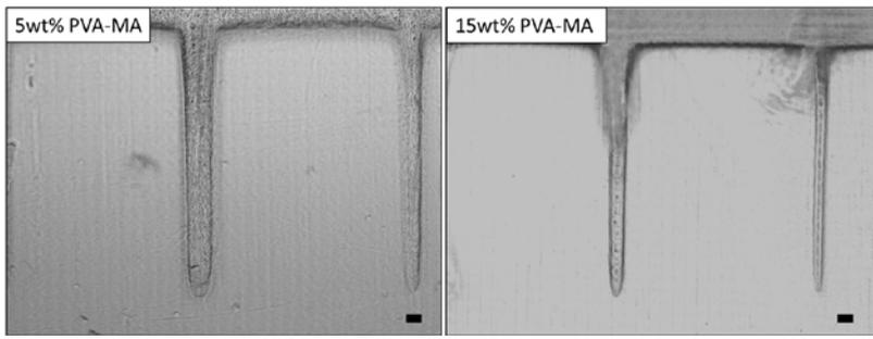
Figure S6: Comb-like structure printed with 5wt% and 15wt% PVA-MA bioresin. Scale bar = 50 $\mu$ m.
