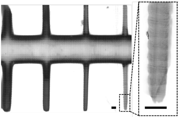
Figure S4: Comb-like structure printed with the PVA-MA/gel-MA bioresin. Scale bar = 50 $\mu$ m.
